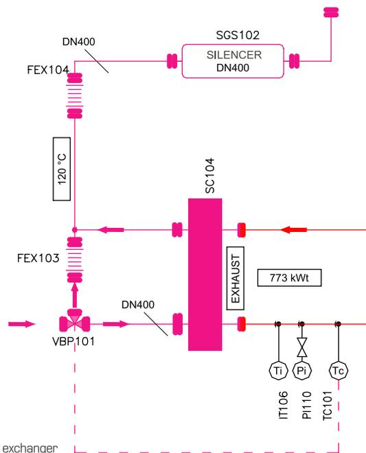
Fig.3 Water exhaust exchanger
