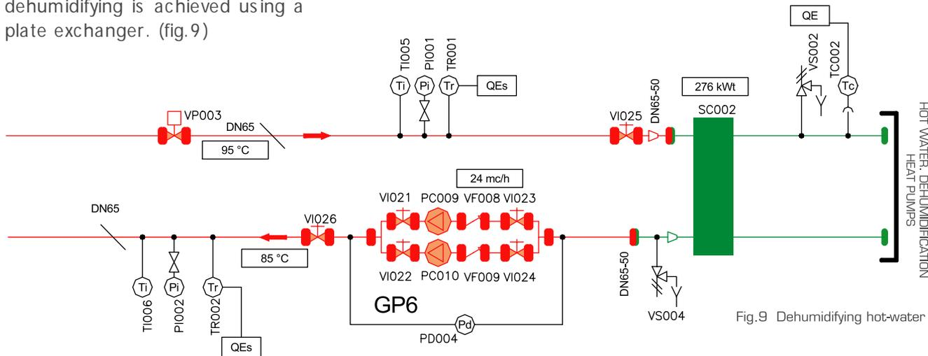
Fig.9 Dehumidifying hot-water circuit
