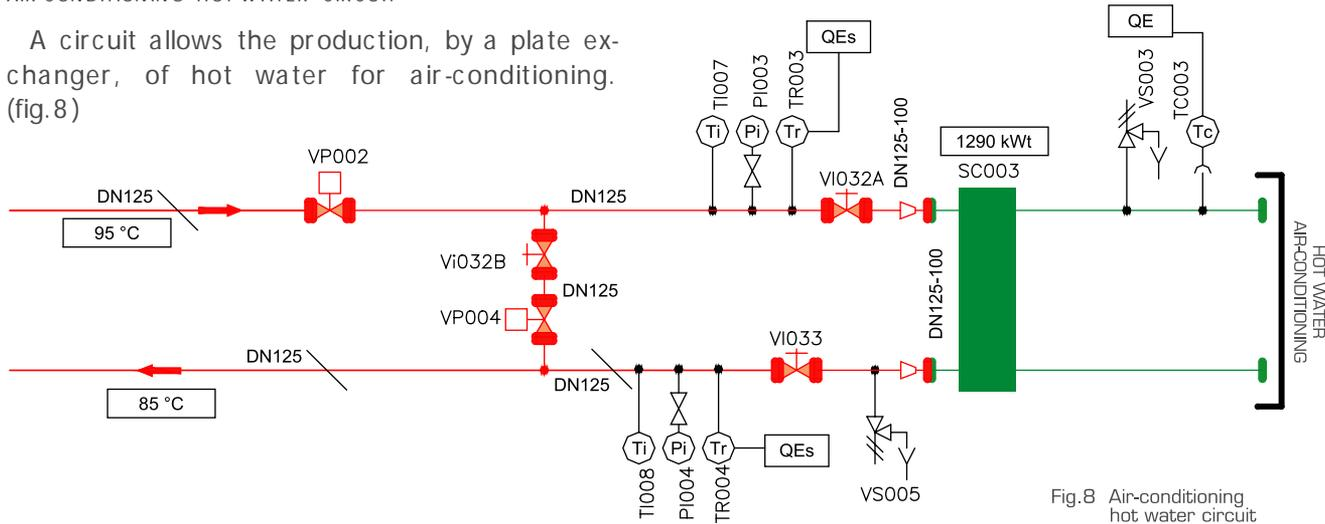
Fig.8 Air-conditioning hot water circuit
