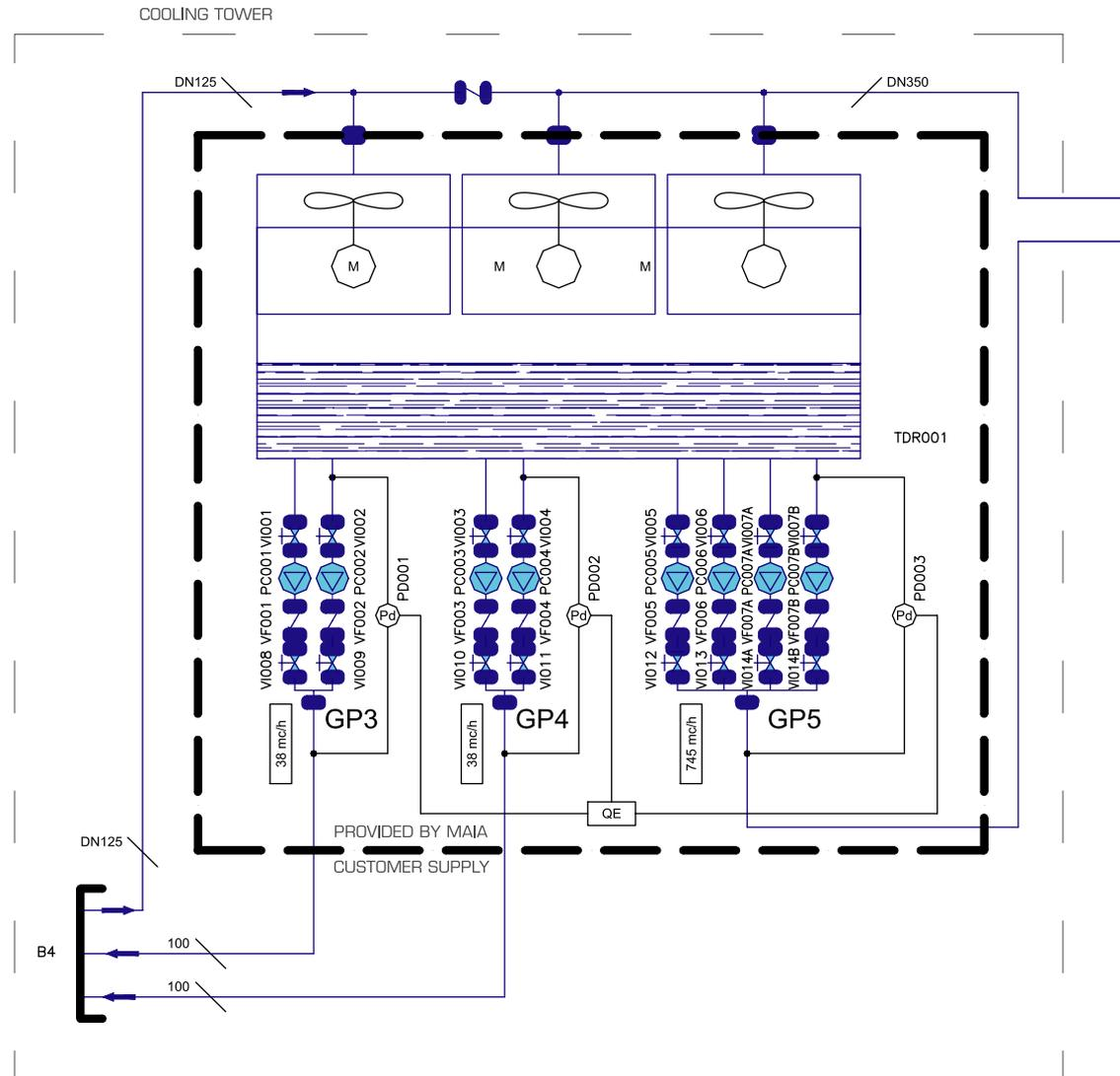
Fig.6 Evaporation tower
